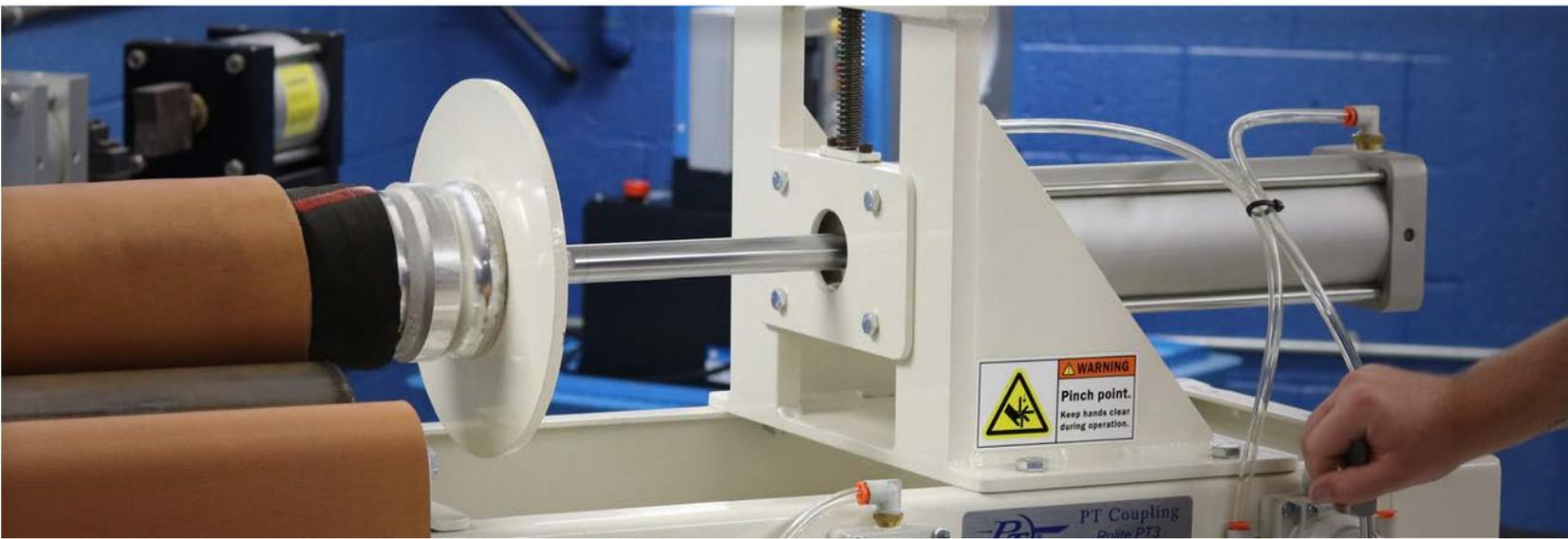
ROLITE PT3 FITTING MASTER is PT's solution for an easy installation and removal of fittings when handling hose assemblies. With pneumatic controls, and manufactured from high quality materials, the Rolite is the simple and cost-effective solution for high production hose assembling.
